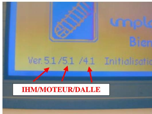
As of version 5.1 of the main implanteo software (IHM), the three software versions appear on the screen in the order IHM / PIC MOTEUR / PIC DALLE
