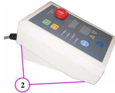
3. Rotate Control Box face plate 90°, being careful not to over extend the ribbon cable.
