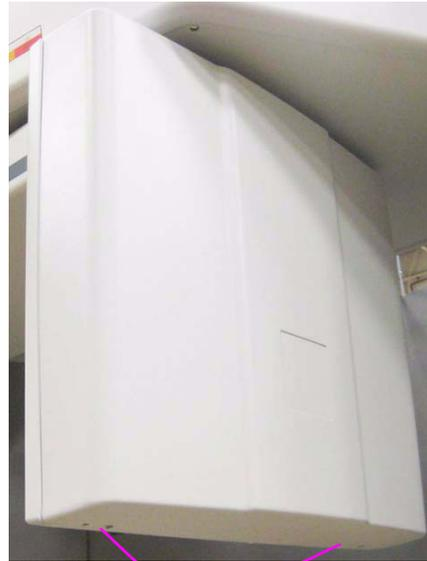
3. On the Receptor Assembly, loosen the two panel mounting screws.
