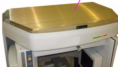
3. Unit must be leveled from side-to-side and front-to-back.
