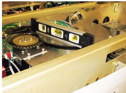
4. Level Overhead Gear using 1/4" Hex Driver to adjust the front Gantry feet.
