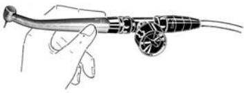
Pict. 2 - Regulating driving air pressure
